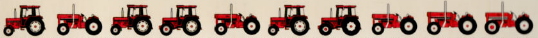
433 26 kW/35 PS V 433 26 kW/35 PS 533 33 kW/45 PS 533 A 33 kW/45 PS V 533 33 kW/45 PS 633 38 kW/52 PS 633 A 38 kW/52 PS V 633 38 kW/52 PS E 633 38 kW/52 PS E 633 A 38 kW/52 PS
