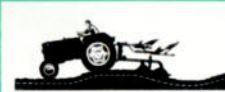
Draft control assures that operating depth is automatically and accurately controlled irrespective of soil conditions.
