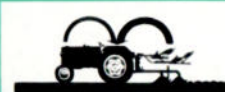
Surplus weight and vertical forces acting on the plow are transferred to rear axle, this gives added traction.
