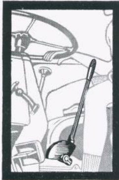
Neutral — Agriomatic lever is in the rear position.
