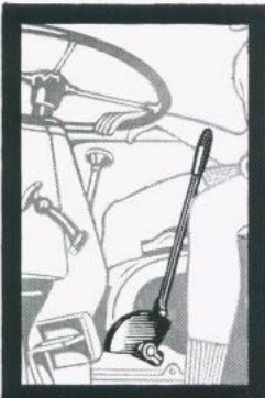
Agriomatic lever is returned to neutral position.
