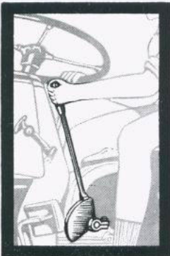
Low range — Agriomatic lever is moved to forward position.
